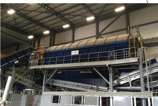
(1) MECHANICAL SCREENER TO SEPARATE DIFFERENT COMPONENTS
